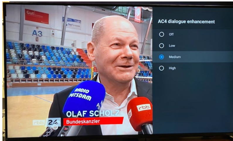
Fig. 9: User interface for Dialogue Enhancement on a Philips DVB-I Prototype TV (page 15) and in a DVB-I application on an Android mobile device (page 16)
